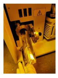
7. Pump down the system: Put cold trap back into the system. Turn "Vacuum" knob to "Vacuum" to start the mechanical pump. The vacuum reading should go down quickly.
