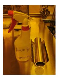
Spray a thin coat of Micro 90 2% solution onto the cold trap and use wipe to clean the liquid.
