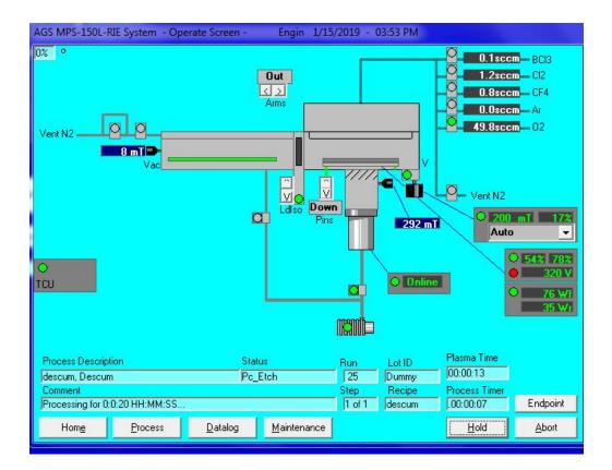
8. Once the recipe is over. The chamber should be vented and ready for unload. Unload your sample and close the cover.
