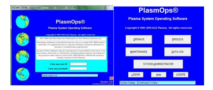
2. Click "operate" at the home page. Ready to load your sample in the loadlock. Turn on the front panel power supply and match controller MC2.
