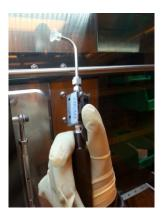
2. Use vacuum wand to load and unload substrate. Adjust the pressure of the glovebox with foot paddles if needed.
