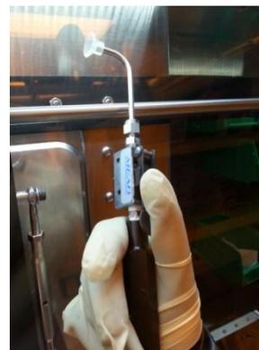
2. Use vacuum wand to load and unload substrate.
