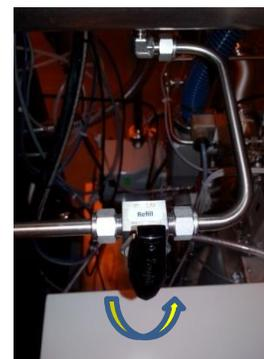
\*Repeat the pump down and refill with N2 to the loadlock for **THREE times!** Foot paddles for “VAC” and “Gas” the glovebox if needed.
