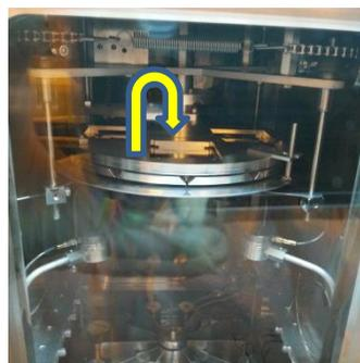
3. Close the door and latch the level. Push the button to seal the chamber door.
